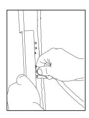
Tuck leads against the acoustic damping material to prevent the wires from touching the back of the speaker surface.
